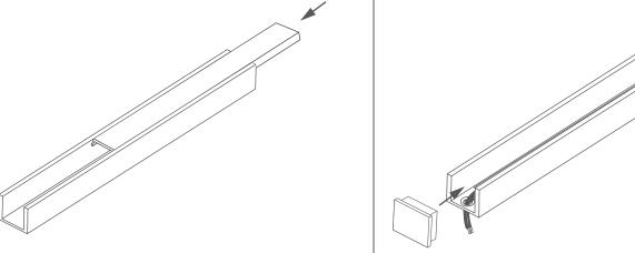
**OPTIONALLY:** The end caps can be attached to the extrusion using glue.
