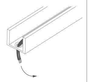
**4.** Connect the LED strips with wires by soldering.
