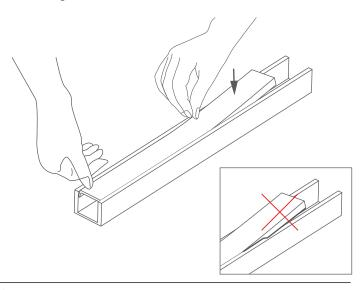
**OPTIONALLY:** Short sections, can also be inserted from the edge of the extrusion.
