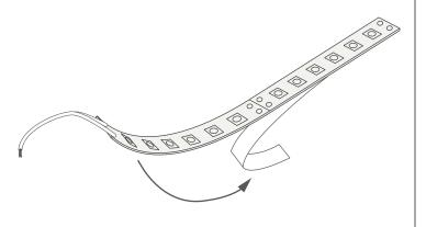
**2.** Attach the tape in the extrusion using the adhesive provided on the LED strip.
