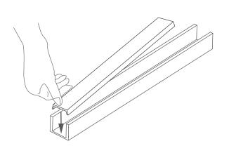
${f 2.}$  Press in the subsequent sections of the cover. Be careful not to bend or break the wings of the cover.
