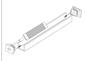
$\boldsymbol{3}_{\bullet}$  Apply a silicone layer to the bottom of the profile and embed the LED strip in it.
